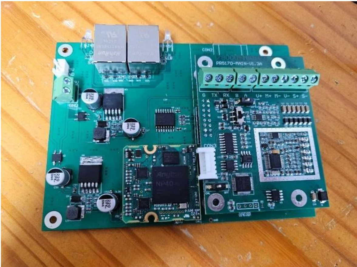
Shared baseboard and analog-input mainboard assembled with an industrial Ethernet module purchased by Minebea Intec.
